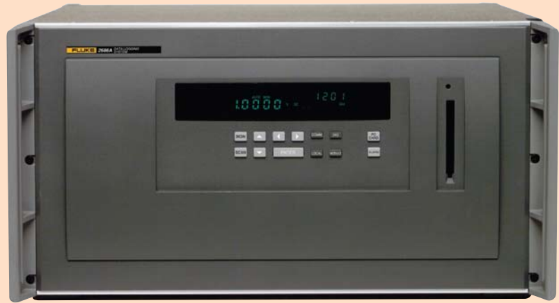
2686A Data Logging System
